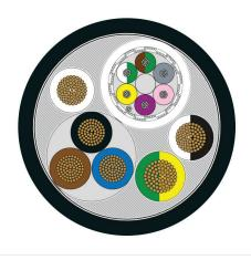
нмс6 Conductor Flexible Tinned copper Polyolefin - Grey, Pink, Violet, Yellow, Insulation
